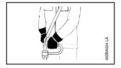
Always hold the brushcutter firmly with both hands. Wrap your fingers tightly around the handles, keeping the handles cradled between your thumb and forefinger. Keep your hands in this position, to have your brushcutter under control at all times. Make sure your brushcutter handles and grip are in good condition and free of moisture, pitch, oil or grease.
