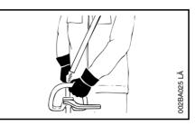
To reduce the risk of bodily injury resulting from loss of control and/or contact with the cutting tool, make sure your unit is equipped with the proper handle and harness for the type of cutting attachment being used (see chart in chapter on "Selecting the Cutting Tool").
